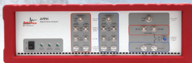
Option LO offers access to internal LO's and individual RF channels
