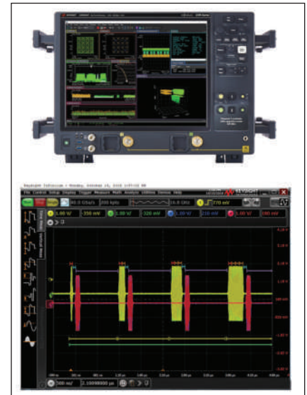
▲ Fig. 8 Real-time scope with display of Rabi oscillation waveforms.
